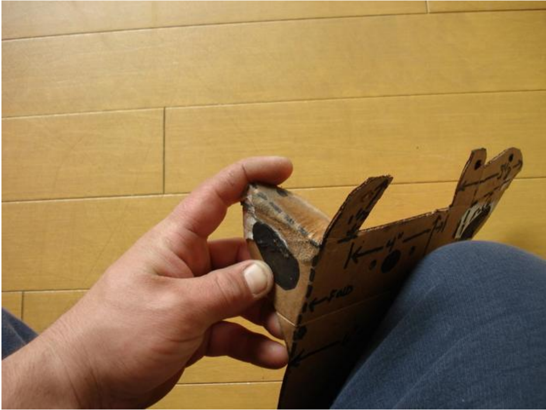
Third picture shows bending the side-light tabs and forward bolt mounts.
